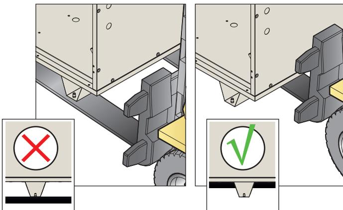
Lift the unit with the forks resting on its bottom, not on the foot brackets
