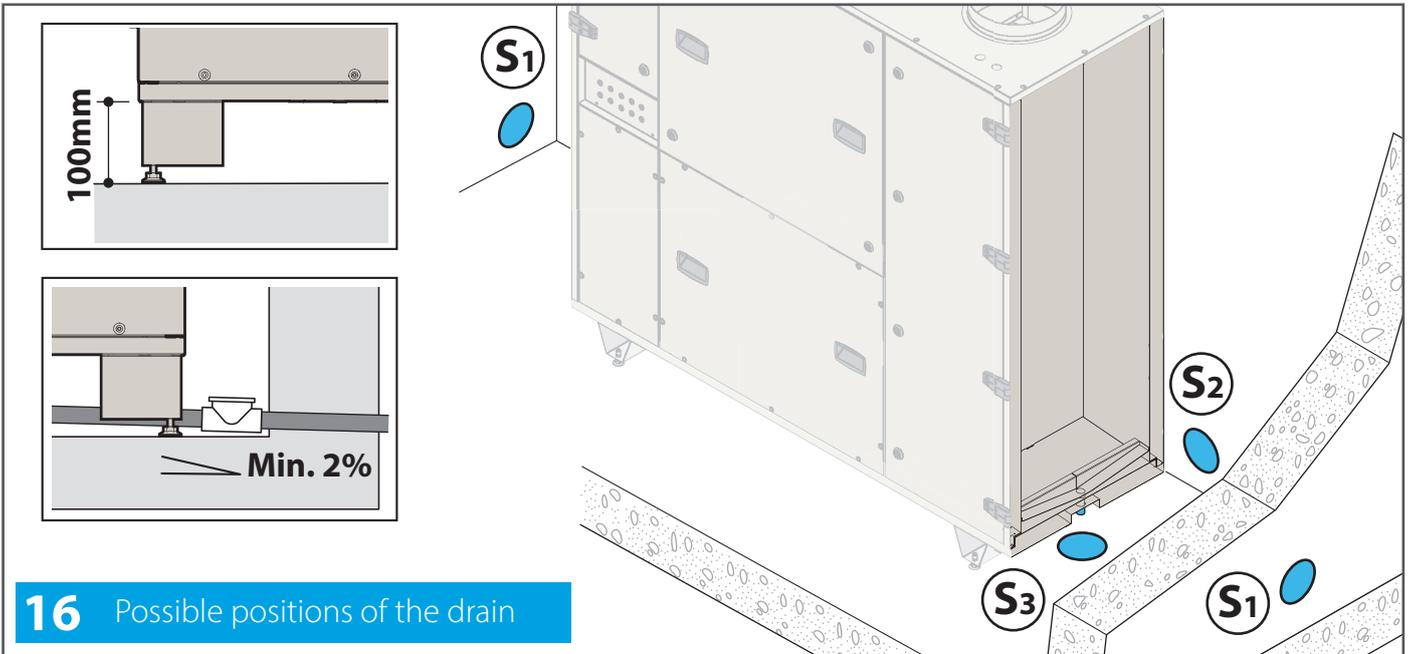
**17** The drain pipe must have a larger diameter than the unit drain (3/4" F) and a minimum inclination of 2% in order to guarantee its operation. In case of wall drain, it is advisable to use a 90MF 3/4" fitting (not supplied) to avoid narrowing in the drain pipe.
