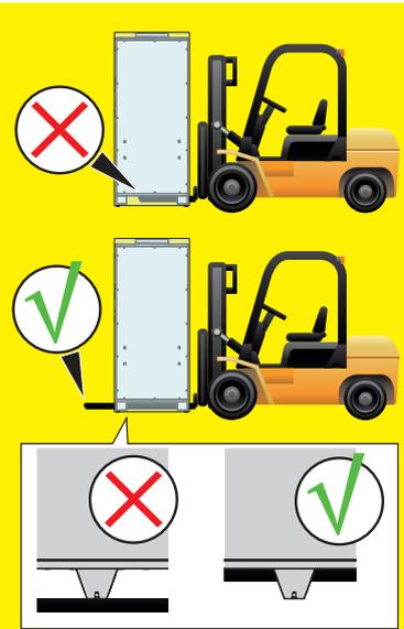
Lift the unit with the forks resting on its bottom, not on the foot brackets
