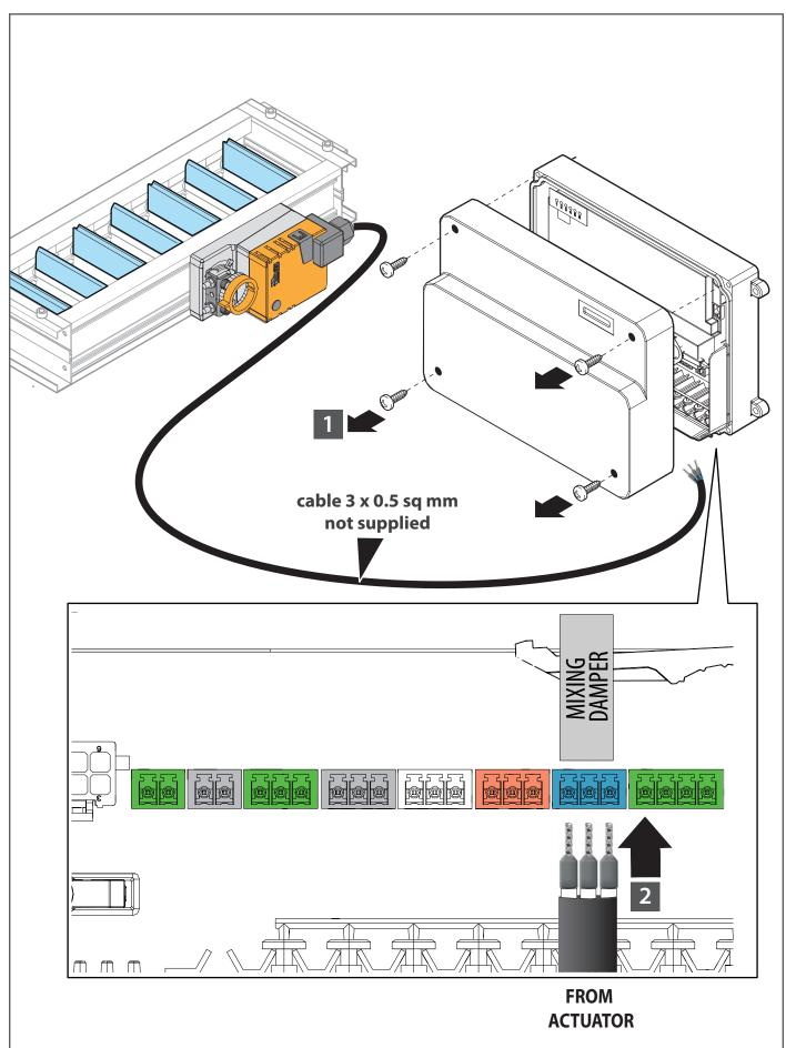
**Connect according to** the wiring diagram
