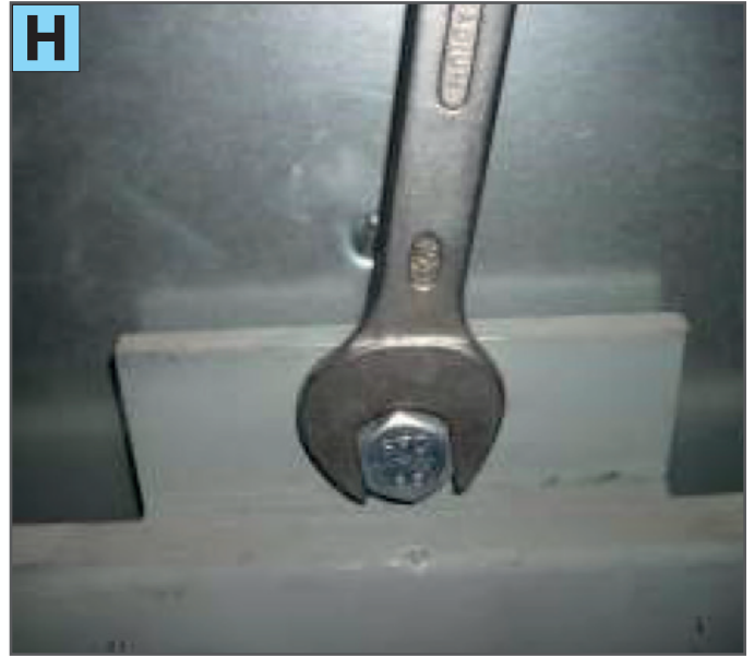
4) Tighten bolt 1 (photo H)
