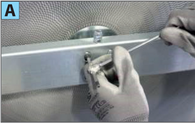
1) Loosen the 4 screws (photo A)
