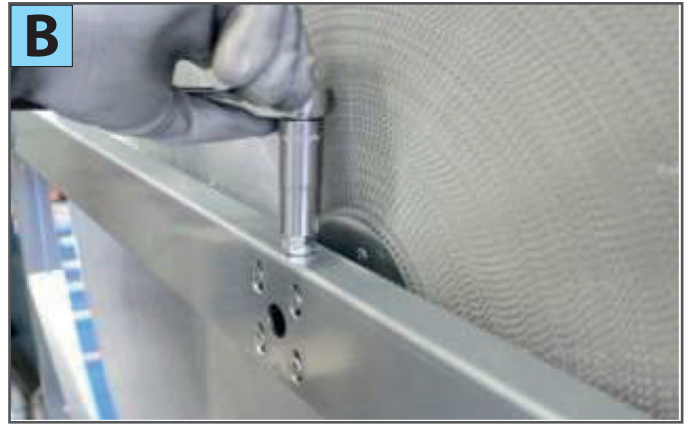
2) Adjust the toe-in of the wheel using the vertical bolt (photo B)
