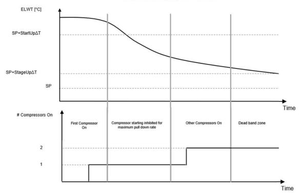
When controlled temperature is within the dead band (DB) error from the active setpoint (AS), unit capacity will not be changed.
