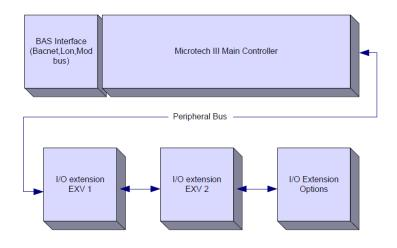
All boards are supplied from a common 24 Vac source. Extension boards can be directly powered by the Unit Controller. All boards can be also supplied by a 24Vdc source.
