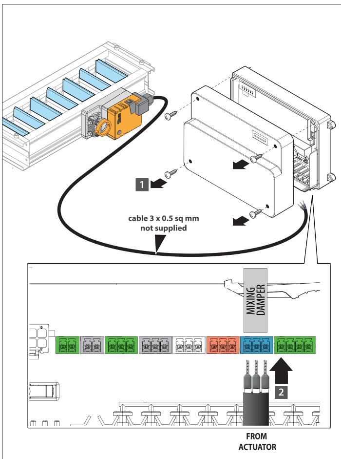
**Connect according to** the wiring diagram
