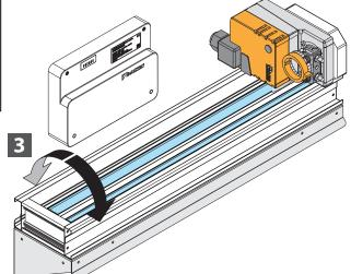
Check if the blades move until completely opened. If blades functioned differently, check the actuator's wiring connection.
