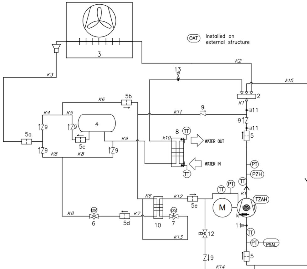
Abbildung 16 - Refrigerant circuit (P&ID) diagram for MONO circuit EWYE-CZ unit
