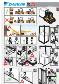
Holes in the base frame not suitable for lifting operations
