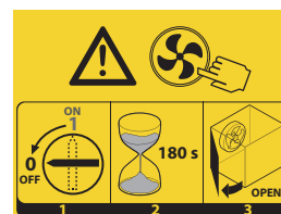
Danger of running fans
