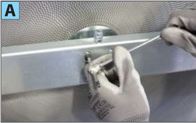
1) Loosen the 4 screws (photo A)
