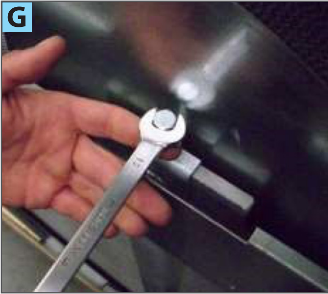
3) Adjust the toe-in of the wheel using screw 2 (photo G)
