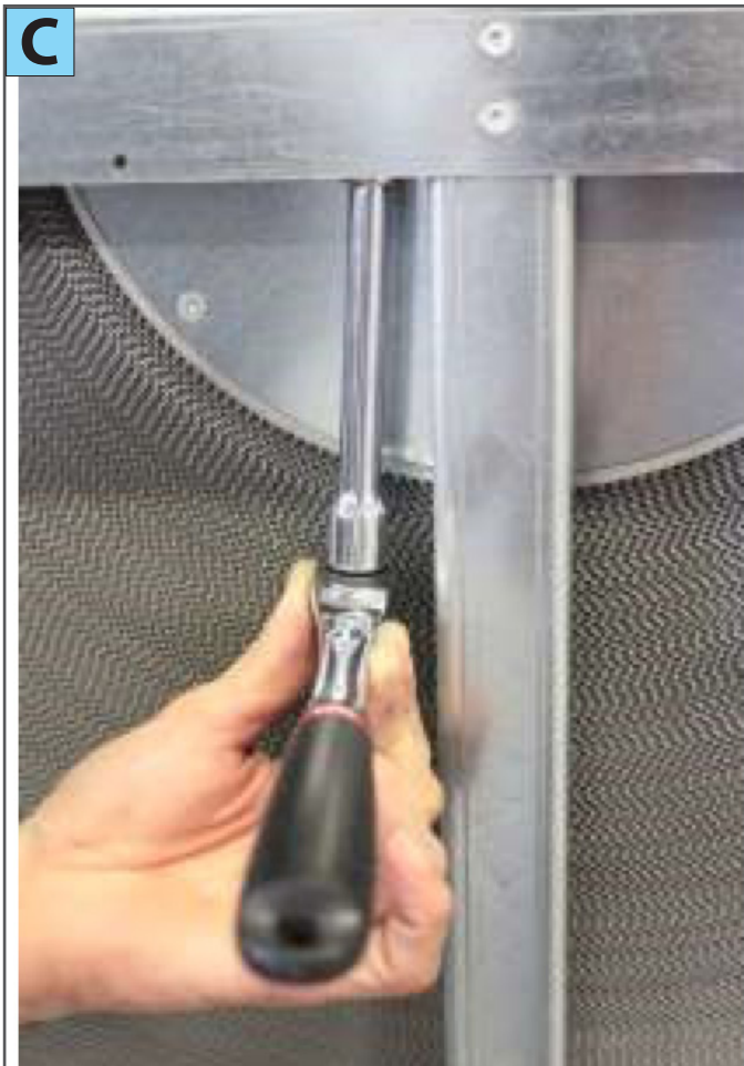
1) Loosen the two screws (photo C)
