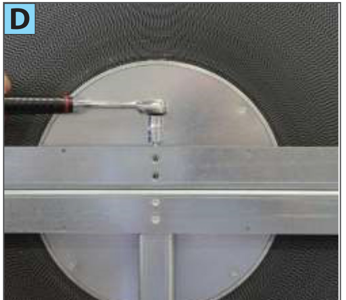
2) Adjust the toe-in of the wheel using a vertical screw (photo D)
