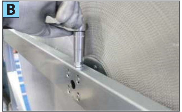
2) Adjust the toe-in of the wheel using a vertical bolt (photo B)
