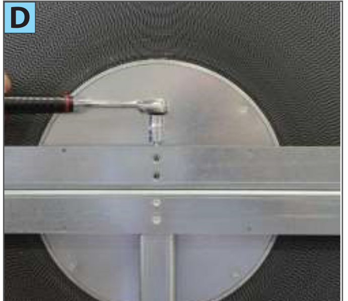
2) Adjust the toe-in of the wheel using the vertical screw (photo D)
