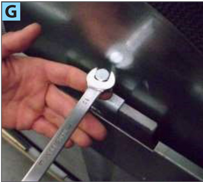
3) Adjust the toe-in of the wheel through bolt 2 (photo G)
