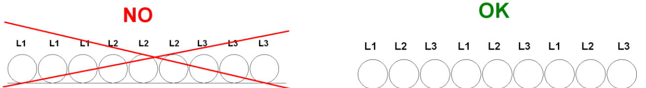
Figure 17 - Installation of long power supply wires
