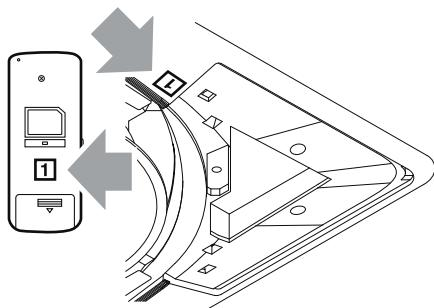
**NOTE** Set the Unit No. of the receiver and the wireless remote controller to be equal. If the settings differ, the signal from the remote controller cannot be transmitted.
