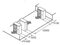
In case of installing multiple units (2 units or more) in lateral connection per row.
