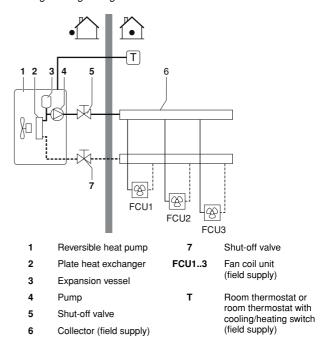
■ Pump operation and heating and cooling (cooling and heating application with a room thermostat suitable for cooling/heating changeover connected to the unit)
