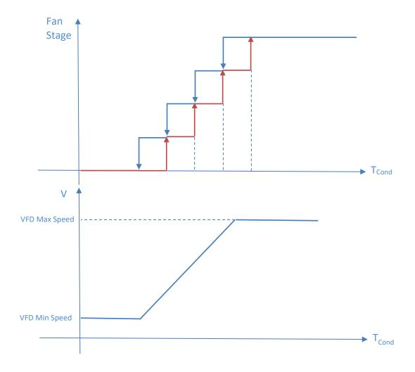
• 1 Vfd by mean of a modulating 0-10V signal generated through a PID controller. The following graph is an example of the modulating signal behavior in case of a PID control supposed to be purely proportional.
