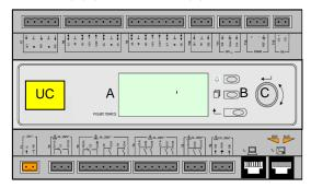
The keypad/display (A) consists of a 5-line by 22 character display. The function of the three buttons (B) is described below:
