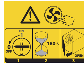
Danger of running fans
