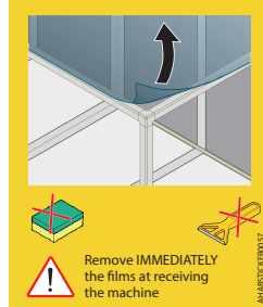
Roof film removal
