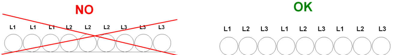
Figure 17 - Installation of long power supply wires
