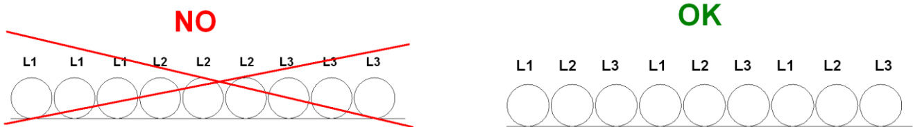
Figure 17 - Installation of long power supply wires
