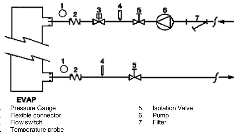
Figure 6 - Water piping connection for heat recovery exchangers
