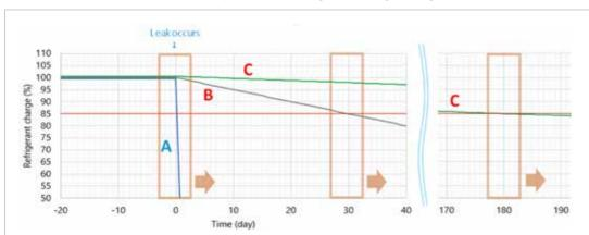
A) Rapid leak: All refrigerant leaks within 1 day - leak speed = 70 kg/day = 25,550 kg/year B) Slow leak 1: 15% of refrigerant leaks in 1-month - leak speed = 0.15 kg/day = 54.8 kg/year C) Slow leak 2: 15% of refrigerant leaks in 6-months - leak speed = 0.025 kg/day = 9.1 kg/year
