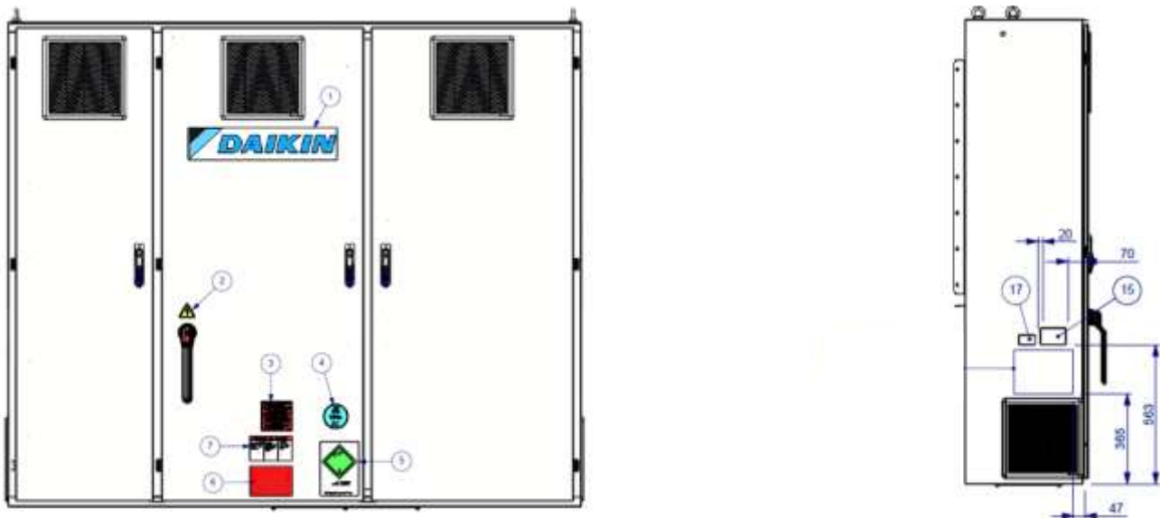
Fig. 29– Description of labels applied on the electrical panel large.
