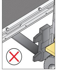
Lift the unit by inserting the forks into the holes provided in the support base
