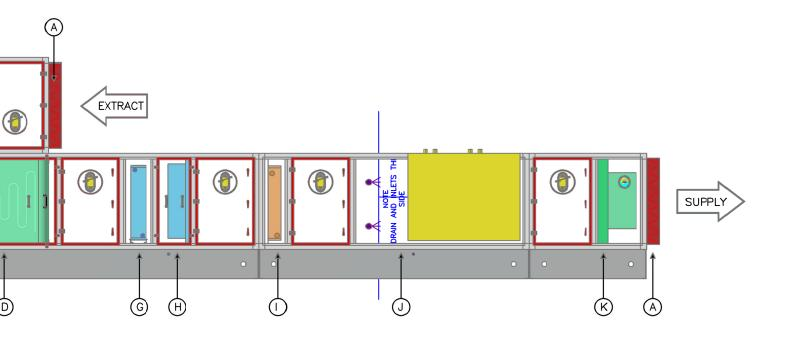
with a minimum fin spacing of 2.5mm. Coils above 1200mm in height will include for intermediate drain trays. All coil mounts & drain pans will be minimum SS316. Access provided both sides of the coil. Drain pans will be fixed with suitable access for maintenance.
