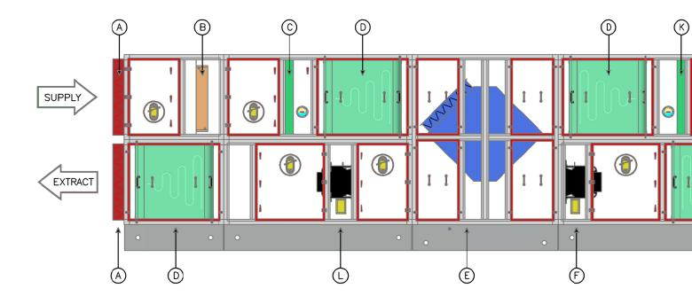
A: Minimum class 3 (BS EN 1751) Aluminium opposed blade low leakage dampers with no plastic parts, suitable for motorisation & included to all openings. Spring return actuators with end switches by others. SS304 & SS316 construction also available.
