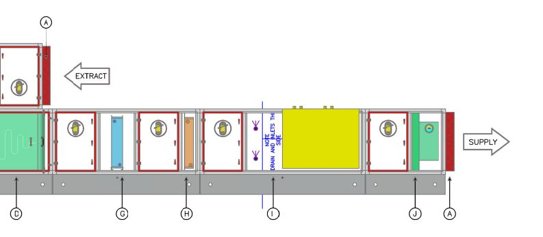
sides of the coil. Drain pans will be fixed with suitable access for maintenance. Slide out moisture eliminator in its own cassette will be provided for applications >2m/s face velocity or where specified (not shown above). All moisture eliminator elements will be minimum SS304 construction. No plastic will be utilised in line with the clause to reduce the use of plastics.
