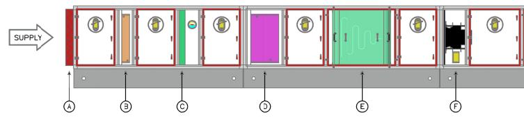
A: Minimum class 3 (BS EN 1751) Aluminium opposed blade low leakage dampers with no plastic parts, suitable for motorisation & included to all openings. Spring return actuators with end switches by others. SS304 & SS316 construction also available.
