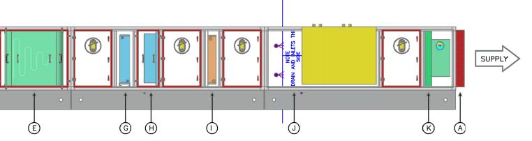
header/copper tube/aluminium vinyl fins/SS304 casing as standard with a minimum fin spacing of 2.5mm. Coils above 1200mm in height will include for intermediate drain trays. All coil mounts & drain pans will be minimum SS316. Access provided both sides of the coil. Drain pans will be fixed with suitable access for maintenance.
